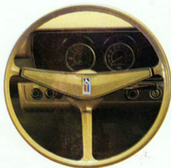
A new instrument panel, with dials deeply recessed to prevent reflections, is standard equipment on all models.
